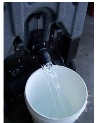
Draining the Recovery Tank
