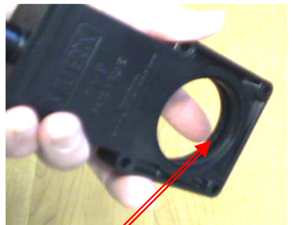
Clean debris from slot in bottom of valve body. Valve slide must be able to slide to bottom.
