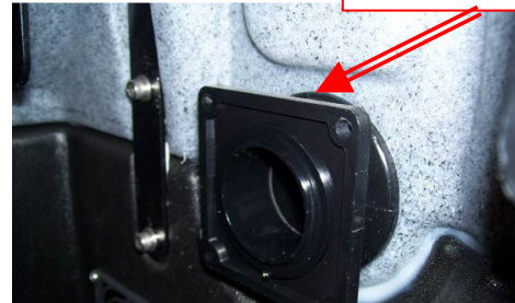
Unless damaged or leaking between tank and flange, the flange fitting does not have to be removed
