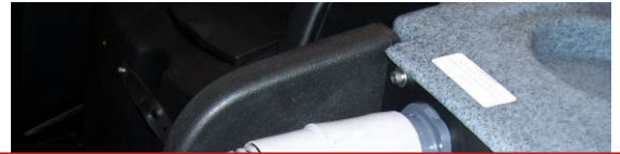
Vacuum Hose Connection with standard barb and vinyl cuff
