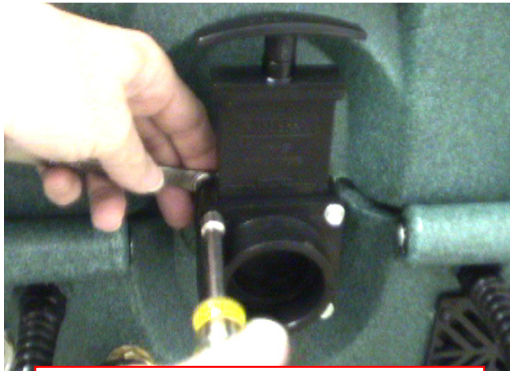
Remove four bolts holding valve assembly to flange fitting
