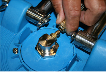
Step 1: Undo the high pressure line at the swivel.
