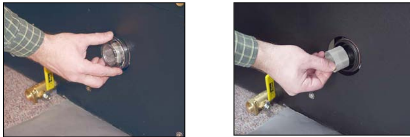
Figure 4-22. Unscrew See-through Cap (Left Photo); Remove and Inspect Filter (Right Photo)
