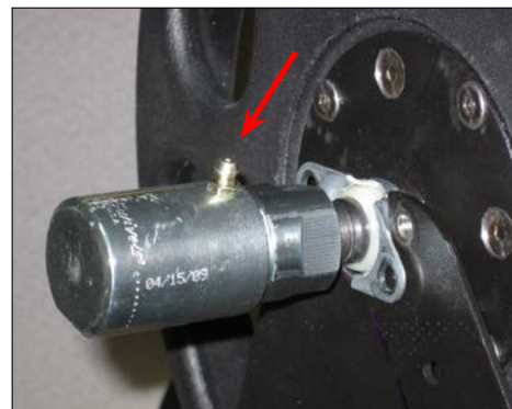
Figure 4-21. Location of Zerk on Swivel
