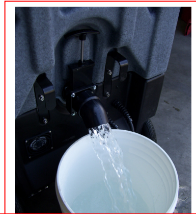
Vacuum acid solution out of Solution Tank
