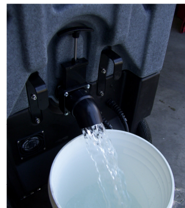
Drain water from Recovery Tank
