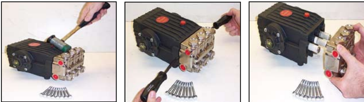
Figure 5-6. Separate Manifold from Crankcase
