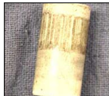
Figure 5-8. Examine Ceramic Plungers
