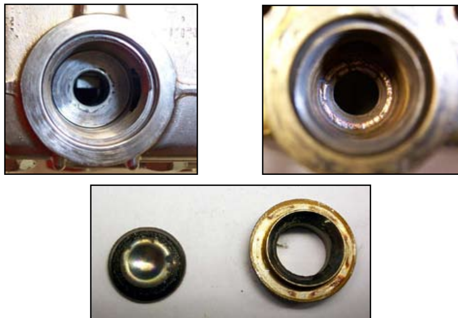
Figure 5-2. Inspect Manifold and Old Valves
