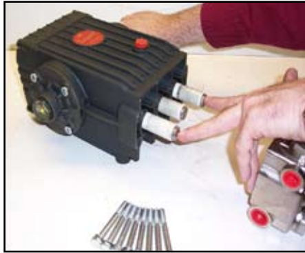
Figure 5-16. Re-install Manifold and Torque Fasteners
