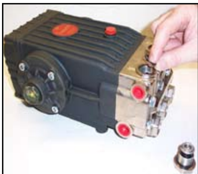
Figure 5-4. Apply Grease and Install Valves
