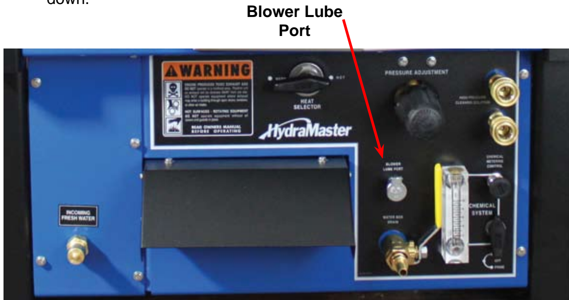
Figure 4-7. Location of Blower Lube Port on Lower Dash Assembly
