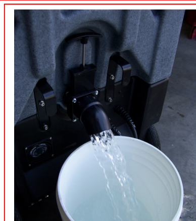
Drain water from Recovery Tank
