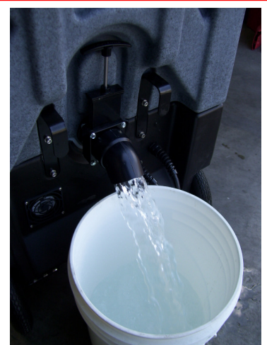
Draining the Recovery Tank
