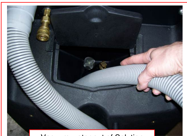
Vacuum water out of Solution Tank
