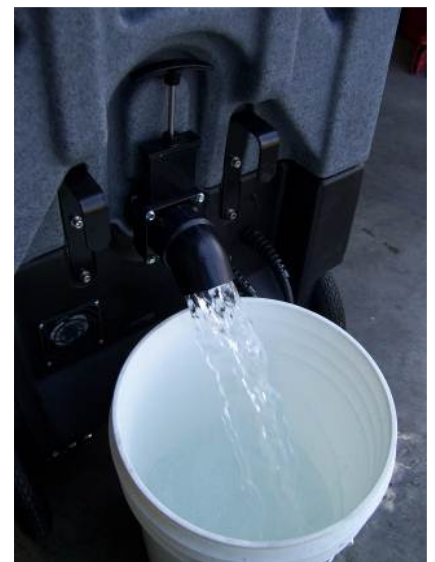
Draining the Recovery Tank
