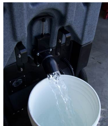
Drain water from Recovery Tank
