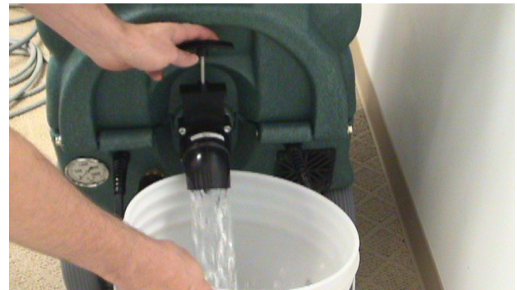
Draining the Recovery Tank
