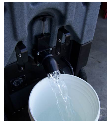
Drain water from Recovery Tank
