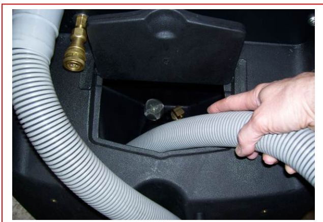
Vacuum water out of Solution Tank
