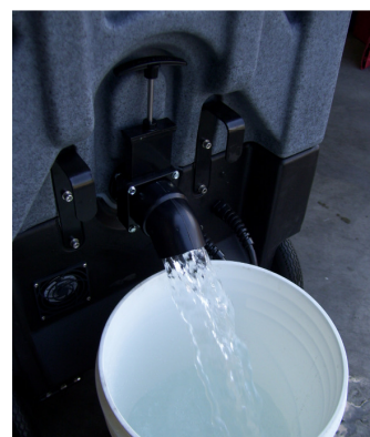
Drain water from Recovery Tank
