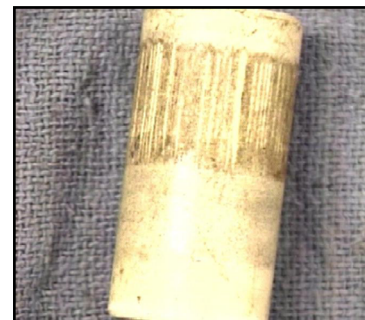
Figure 5-8. Examine Ceramic Plungers
