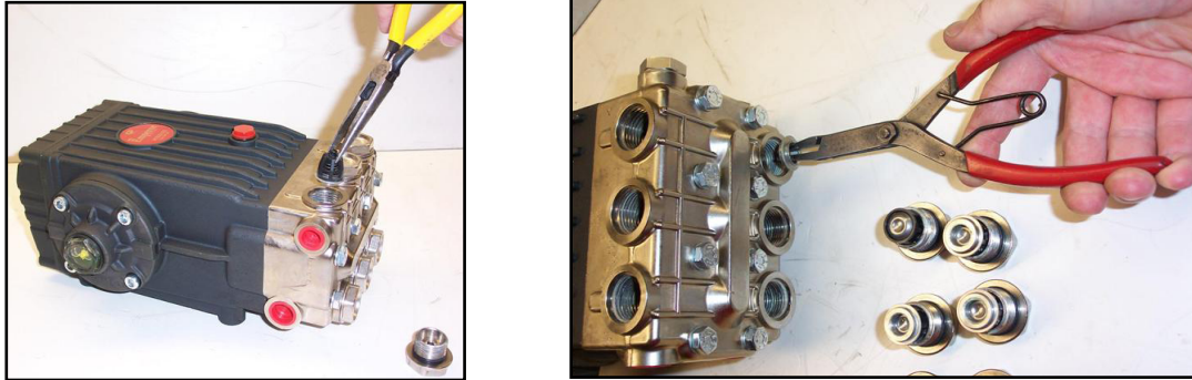
Figure 5-1. Remove Valve Cap and Valve Assembly
