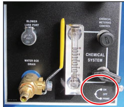
Figure 4-6. Location of Chemical System Switches
