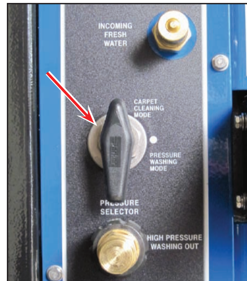
Figure 4-5. Location of Water Pressure Selector Valve (Labels Shown as Part of the High Pressure Washing Kit - P/N 000-079-126)
