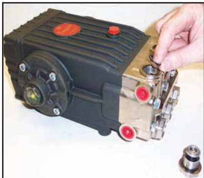
Figure 5-4. Apply Grease and Install Valves
