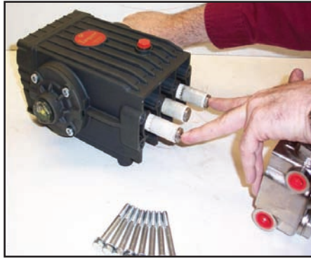
Figure 5-16. Re-install Manifold and Torque Fasteners
