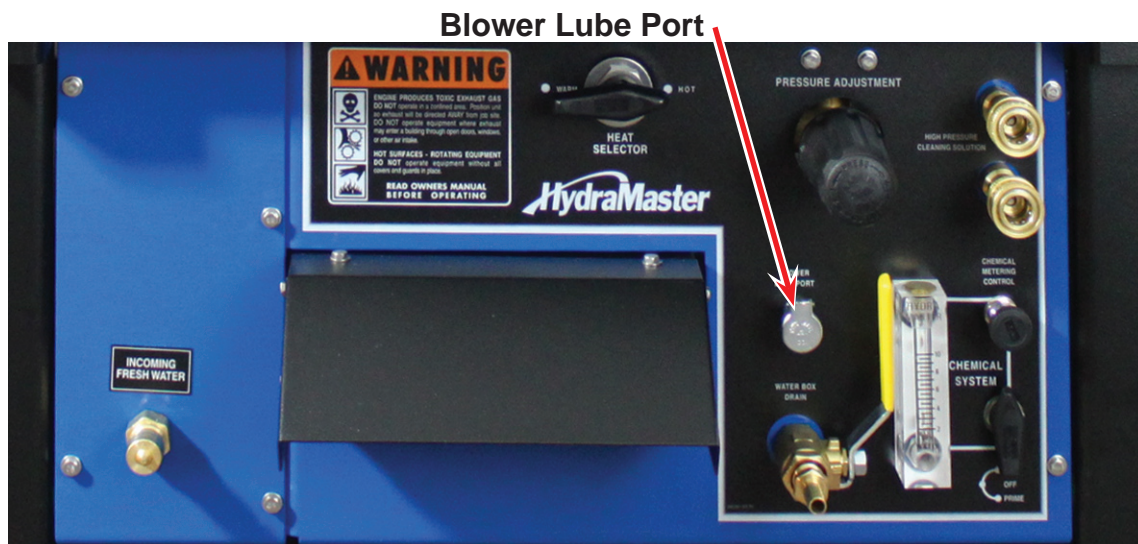
Figure 4-7. Location of Blower Lube Port
