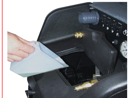
Add appropriate amount of chemical to water in solution tank
