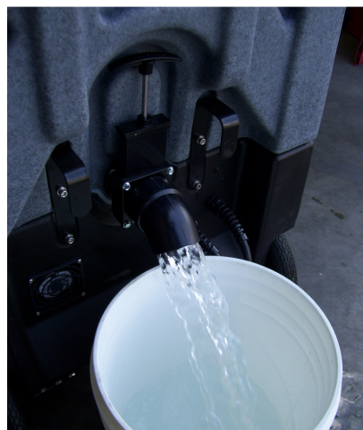
Drain water from Recovery Tank
