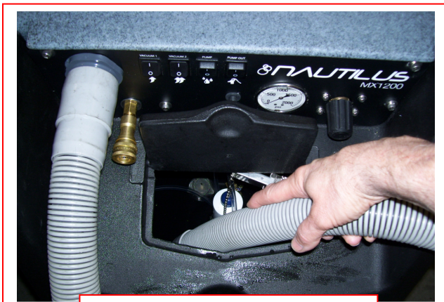
Vacuum water out of Solution Tank
