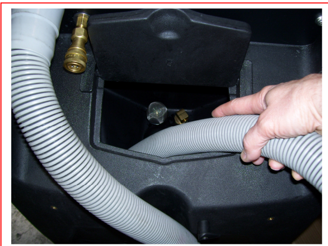
Vacuum water out of Solution Tank
