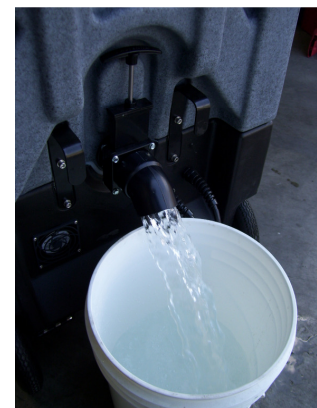
Drain water from Recovery Tank
