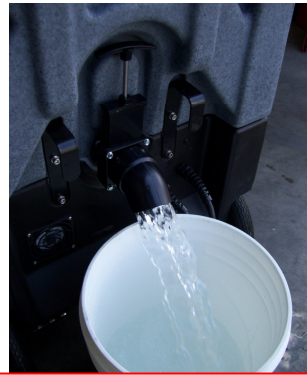
Drain Recovery Tank
