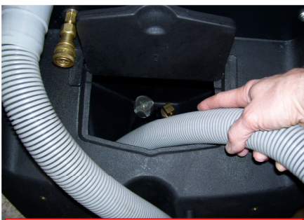
Vacuum acid solution out of Solution Tank
