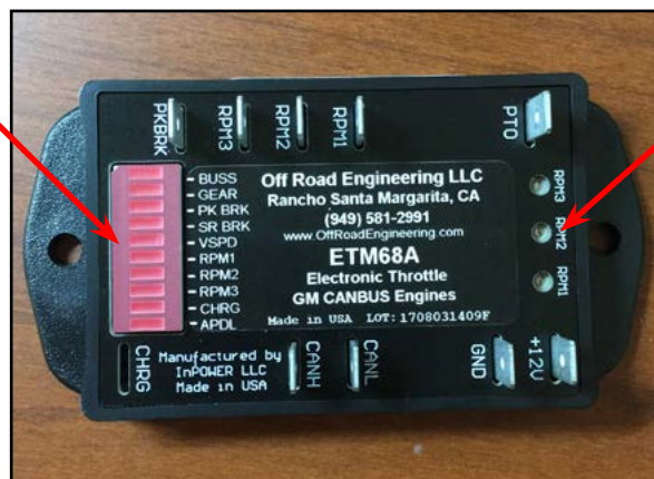
Figure 3-1. Location of Controller’s LED Lights with Labels and RPM Trim Potentiometers
