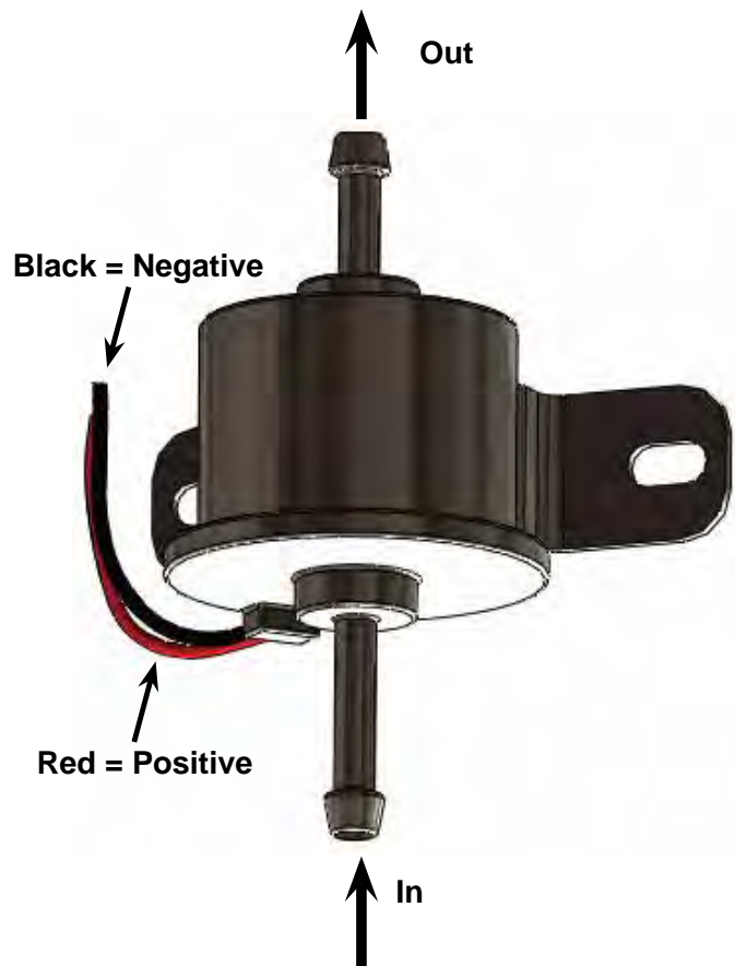
Figure 2-3. Install Fuel Pump, Outlet Side Up
