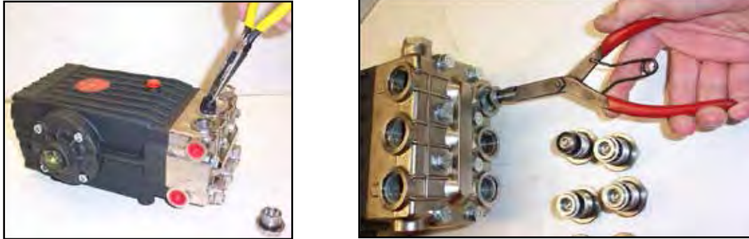
Figure 5-1. Remove Valve Cap and Valve Assembly
