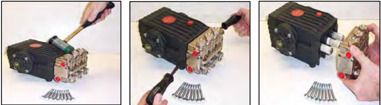
Figure 5-6. Separate Manifold from Crankcase
