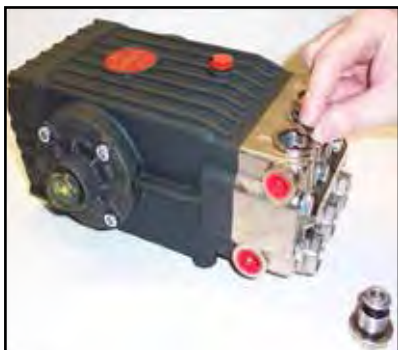
Figure 5-4. Apply Grease and Install Valves
