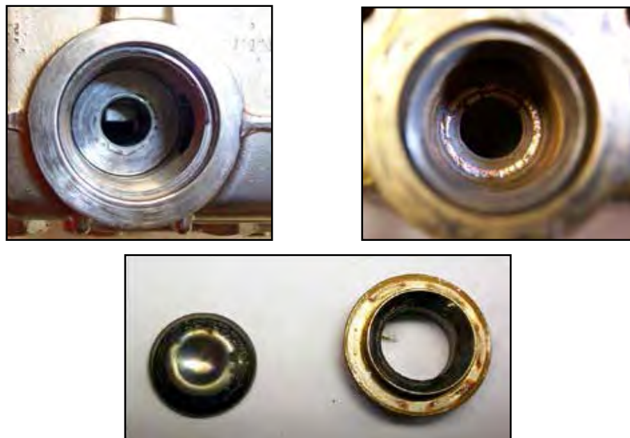
Figure 5-2. Inspect Manifold and Old Valves
