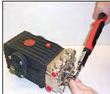
Figure 5-18. Torque Bolts to 22 ft. lbs
