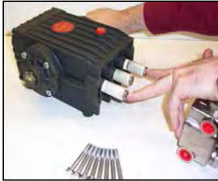
Figure 5-16. Re-install Manifold and Torque Fasteners
