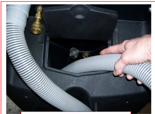
Vacuum water out of Solution Tank
