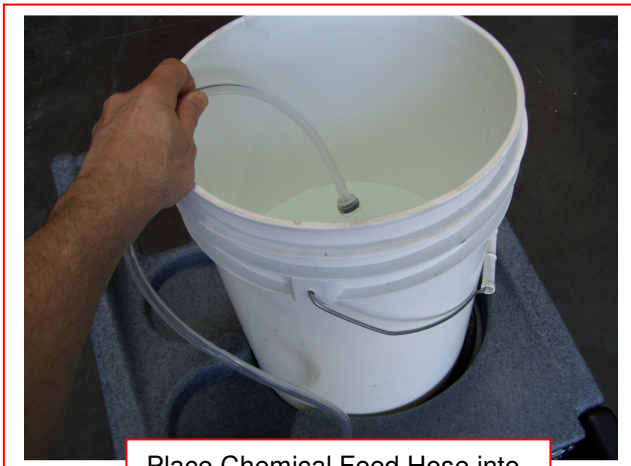
Place Chemical Feed Hose into Rinse Solution
