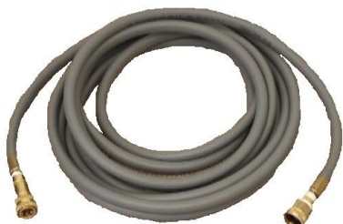
Connect the Auto-Fill Water Supply Hose to Solution Inlet (Male quick connect on the front of the machine.) 3/8" id X 25' with F Quick Connect & F Garden Hose Fitting
