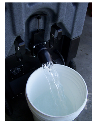
Drain water from Recovery Tank
