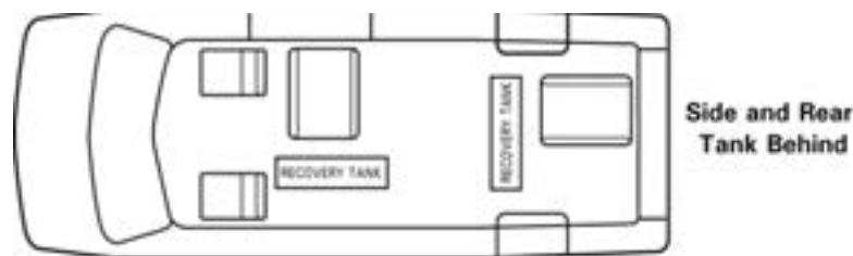
Figure 2-2. Recommended Location of Boxxer 318HP in Van
