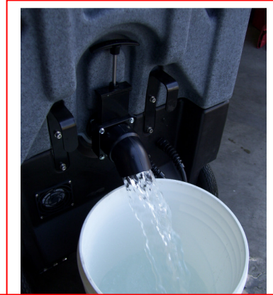
Drain Recovery Tank
