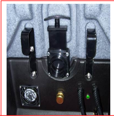
Remove four bolts holding valve assembly to flange fitting
