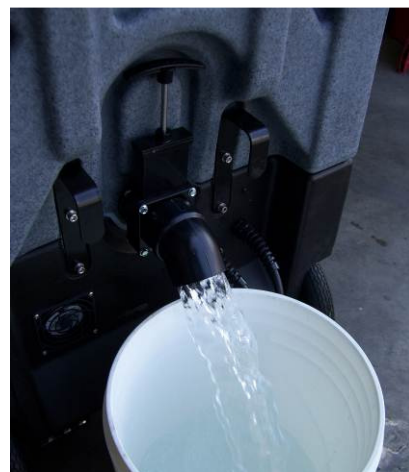
Drain water from Recovery Tank
